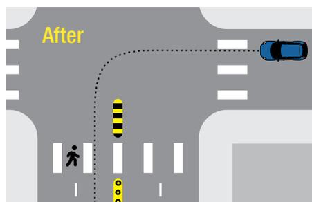
Centerline hardening makes intersections safer for pedestrians by encouraging drivers to make left turns at slower speeds. Bollards and rubber curbs block the diagonal path through the intersection.
