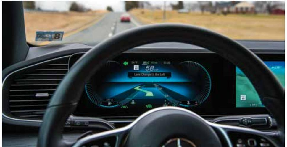
vehicles today is Level 2. These systems continuously control acceleration, braking and steering to keep the vehicle traveling at a set speed in the center of its lane while maintaining a selected following distance from the vehicle ahead. They require the human driver to remain vigilant and ready to intervene in the event that the system encounters a situation it cannot handle.
